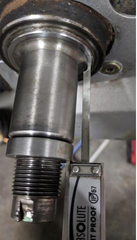
7. Slide the adapter sleeve over the spindle and threaded support ring. NOW - since you likely won't have to touch these for quite a while! - apply a thin layer of anti-seize or high temp grease applied on the spindle beforehand to help later removal/servicing. The sleeve can be tight, just make sure it's straight and install it over the support ring. If it seems too tight please contact us.
