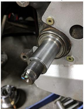
8. Install the pre-assembled hub unit onto the spindle over the adapter sleeve, careful not to force it. Align the bearing and it will slide on and fully seat onto the end of the spindle similar to stock.
