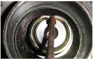
11. Install a new OEM Mazda dust cap per normal procedure. The new bearing cartridge has a metal dust "shield" on the outboard side of the cartridge, but it is not a watertight rubber seal like what's used on the inboard side. It is important to continue using the OEM dust cap to stop water and debris from entering the bearing.
